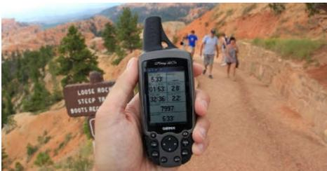
A GPS (Global Positioning System) device is a hand-held receiver that picks up signals from satellites circling the earth, enabling you to locate your current position to an accuracy of 10-20m. Most modern GPS devices can then show that position on a map and, if you have stored a pre-programmed route, help you navigate along it.
